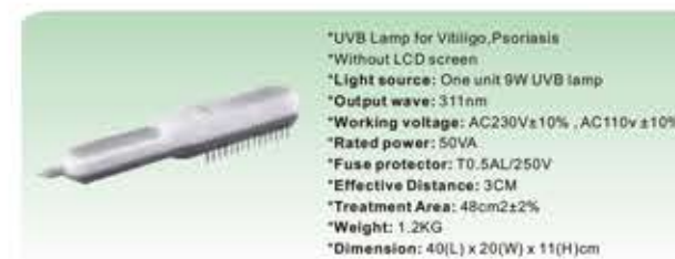
*UVB Lamp for Vitiligo,Psoriasis *Without LCD screen *Light source: One unit 9W UVB lamp *Output wave: 311nm *Working voltage: AC230V±10% , AC110V±10% *Rated power: 50VA *Fuse protector: T0.5AL/250V *Effective Distance: 3CM *Treatment Area: 48cm2±2% *Weight: 1.2KG *Dimension: 40(L) x 20(W) x 11(H)cm MY-S001 UV Radiation Treatment System
